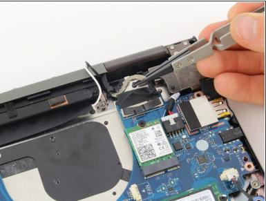
Pull up on the thick gray display cable near the back of the laptop to disconnect the display.
