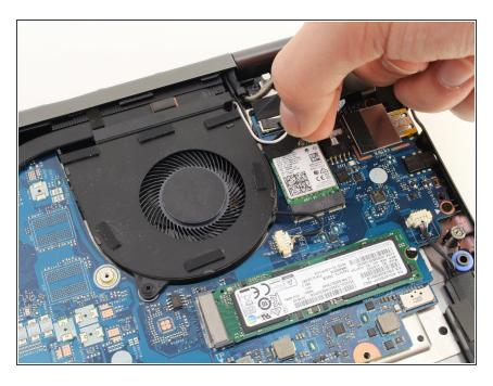
Remove the sticky tape from the top of the wireless card.
