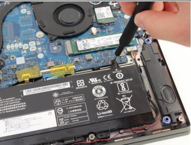
Remove the four 4mm Phillips #1 screws securing the battery.
