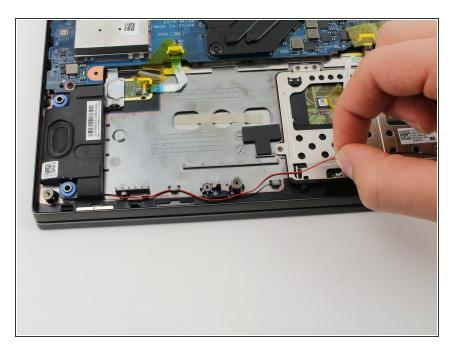
Remove the red and black wire near the front of the laptop from underneath the hooks that hold it in place.
