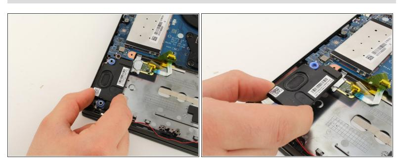
Pull up on the left speaker to remove it from the chassis.
