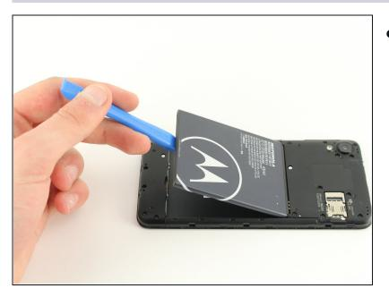
• Use the opening tool on the divot located below the battery to pop it out.
