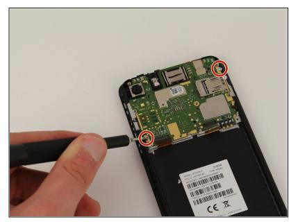
• Remove the two 1.1 mm T4 Torx screws from the bottom left and top right sides of the motherboard.
