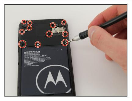
• Remove the eleven 3.8 mm T4 Torx screws located above the battery compartment.
