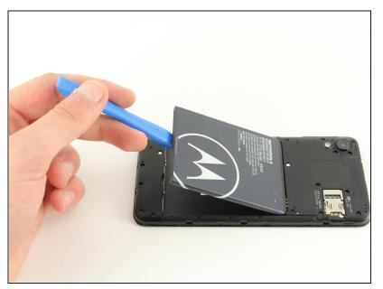
Use the opening tool on the divot located below the battery to pop it out.
