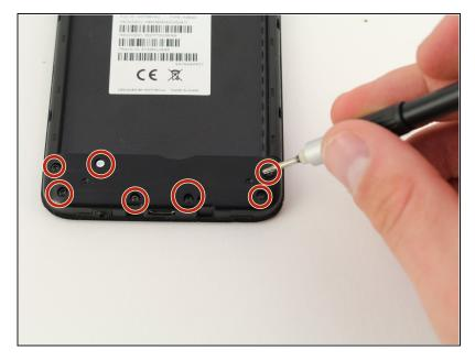
Remove the seven 3.8 mm T4 screws on the piece located below the battery compartment.
