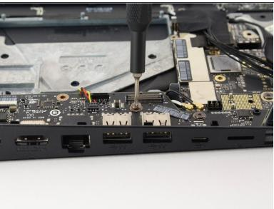
Remove the three T6 Torx screws from the I/O board.
