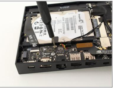
Remove the screw on the metal piece using a T6 Torx screwdriver and put away the metal piece after removing the screw.
