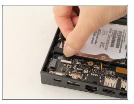
Next to the empty socket where the black wires were attached to the I/O board (refer back to Step 2), detach the plastic strap from the I/O board by pushing the strap away from the socket using your finger.
