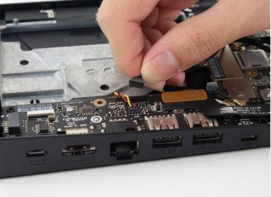
Detach the small bundle of black wires from the I/O board by gently pulling upward.
