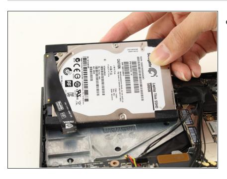
Gently pull the hard drive out of the device.
