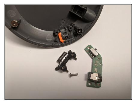
Three more T6s secure a board bringing power input and a microphone switch down the ribbon cable.
