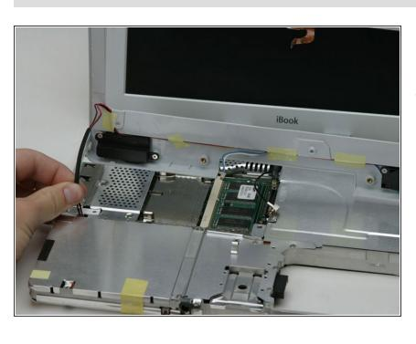
Lift the upper case off completely and disconnect the red and black speaker cable from the logic board. As before, make sure you're pulling only on the connector and not on the socket.
