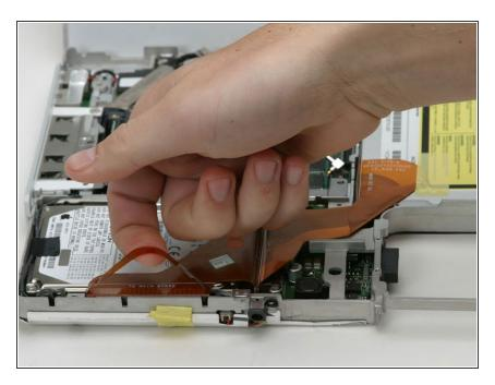
Use the transparent orange loop to disconnect the large orange ribbon cable from the logic board.
