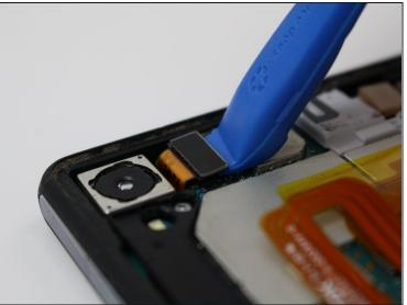
Using the plastic opening tool, carefully pry off the flex connector beside the camera housing.
