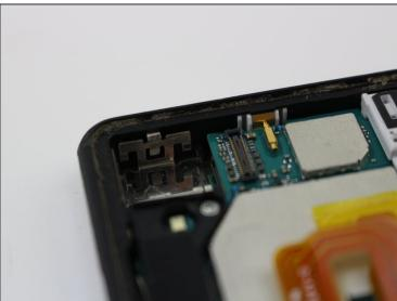
• Use the <u>tweezers</u> to pull the camera out of the top left corner of the phone.
