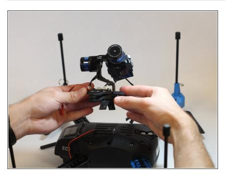
Remove the gimbal mount from the body of the drone.
