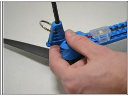
Slide the leg foot out of the leg assembly.
