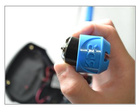
To remove the motor assembly, pull the motor assembly through and out of the leg chassis.
