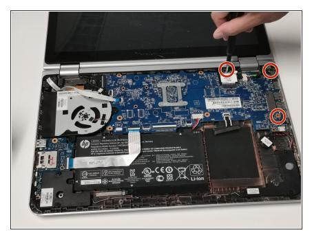
Remove the three 4.5mm Phillips #1 screws from right side of the motherboard.
