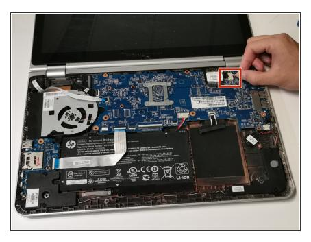
Detach the cable between the CPU and the motherboard.
