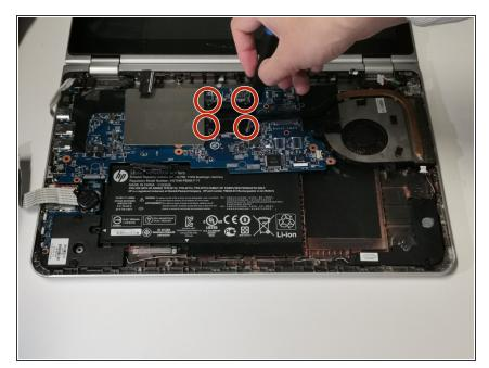
Turn the connected motherboard and fan upside down and remove the four 4.5mm Phillips #1 screws from the middle of the back of the motherboard.
