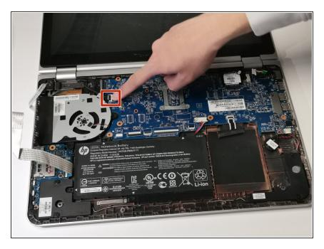
Detach the connection between the fan and the motherboard.
