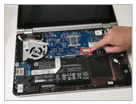
Detach the cable between the battery and the motherboard.
