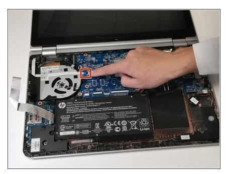
Disconnect the cable between the screen and the motherboard.
