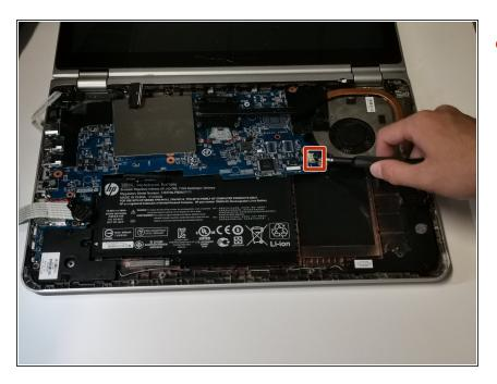
Disconnect the cable connecting the fan to the motherboard.
