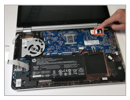
Disconnect the cable between the CPU and the power interface.
