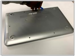
Remove the screw covers using an iFixit opening tool.
