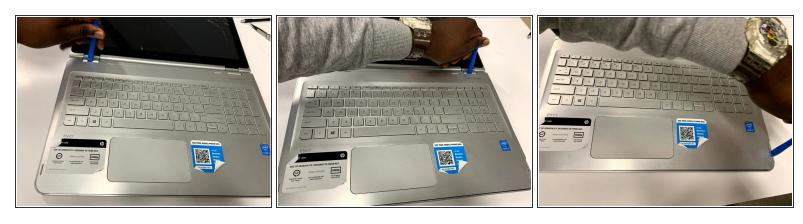
Pry open a gap in the edge of the keyboard with an iFixit opening tool.
