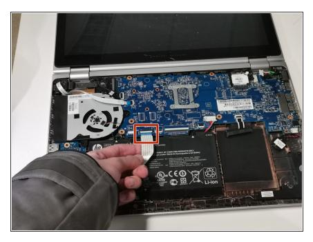
Disconnect the cable between the SD card and the motherboard.
