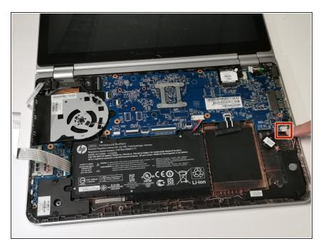
Disconnect the cable from the speaker to the motherboard.
