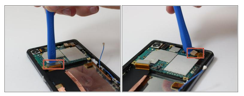
Using an opening tool, disconnect the two press fit connectors from the bottom and top right of the motherboard.
