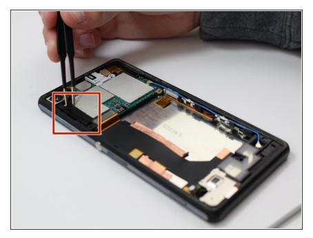
Remove the bracket on the left side of the motherboard with a pair of tweezers.
