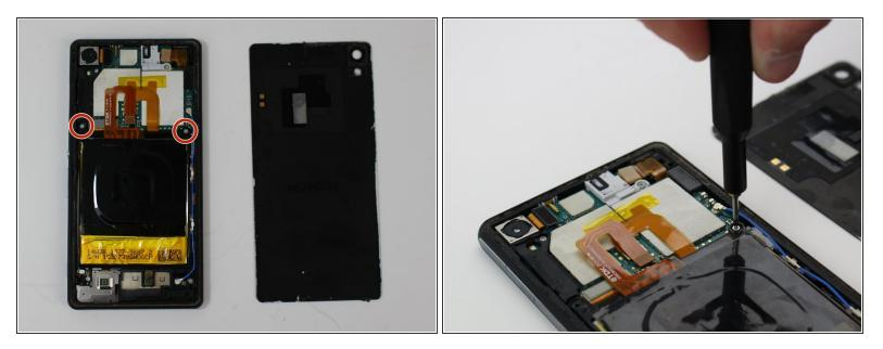
• Use the Torx T5 screwdriver to remove the two 3.81mm screws from the corners of the battery.
