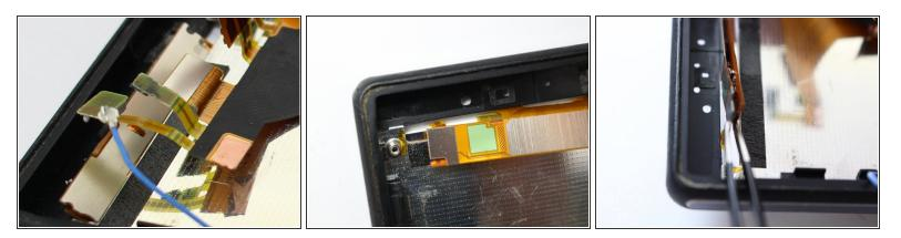
• Turn your attention back to the inside of the device, where there is one group of cables connected to the display on the front of the phone. Maneuver these cables, as shown, through the hole so that the screen and cables can be removed from the device. The screen and attached cables will now detach from the phone.
