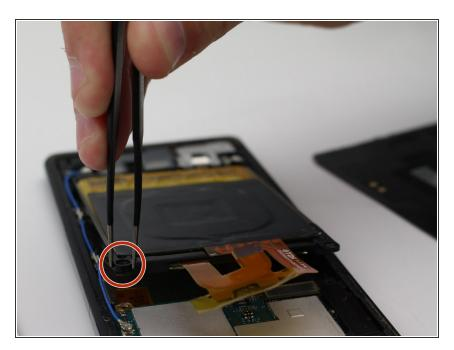
Use the tweezers to grab the top right corner of battery and carefully lift it up and away from the phone.
