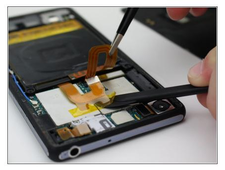
Slowly slip the halberd spudger underneath the rest of the orange flex cable to carefully peel the adhesive portion away from the rest of the phone.
