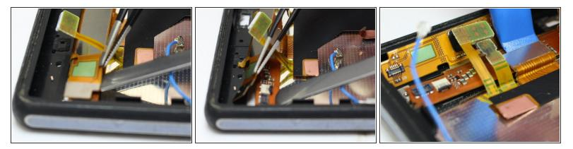
• Disconnect all of the press fit connectors from the circuit board beneath the daughterboard using a plastic opening tool.
