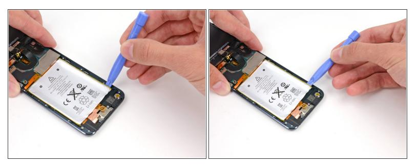
Continue with the lower right notch. Insert the plastic opening tool into the notch, and gently pry up on the side of the battery.
