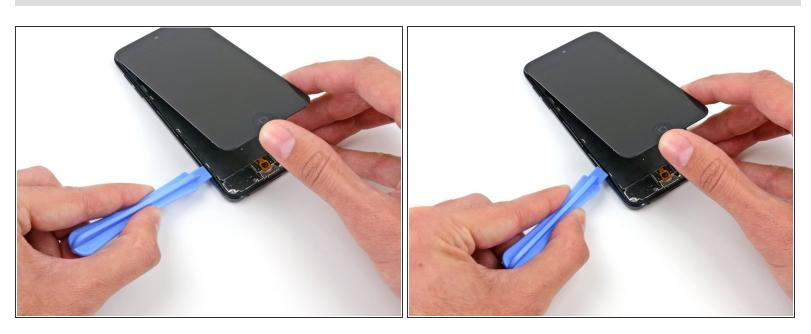
Using the same procedure, loosen the last clip securing the plastic frame to the rear case.
