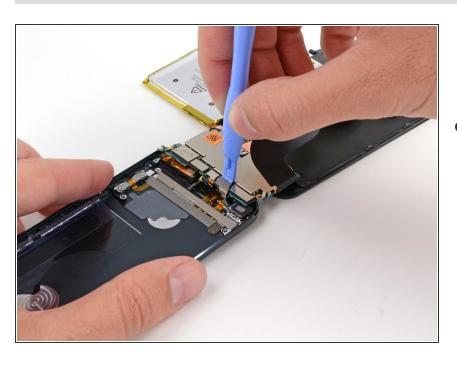
Use the edge of a plastic opening tool to disconnect the rear-facing camera ribbon cable from the back of the logic board.
