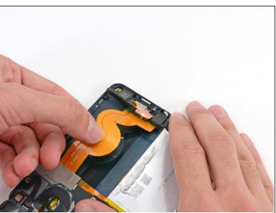
Grasping the large ribbon cable, gently pull the Lightning connector assembly out of the bottom of the case.
