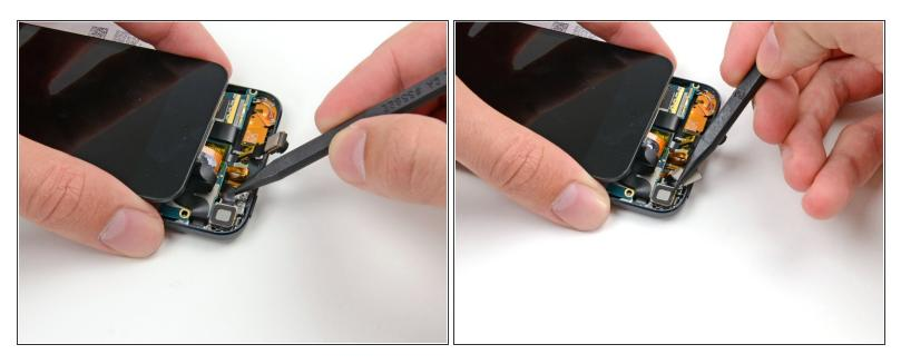
Use the tip of a spudger to gently pull the rear-facing camera ribbon cable out from underneath the logic board.
