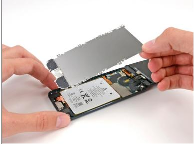
Lift up and remove the LCD plate from the iPod.
