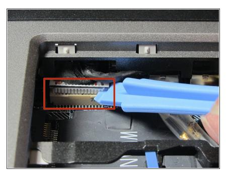
Using the spudger, unhook the touchpad's ribbon cable from the left side of the board indicated in the picture.
