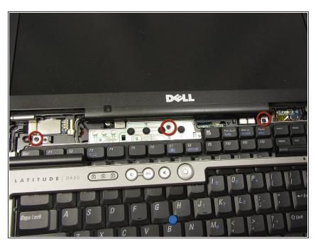
Remove the three 3mm Phillips #0 screws securing the keyboard.
