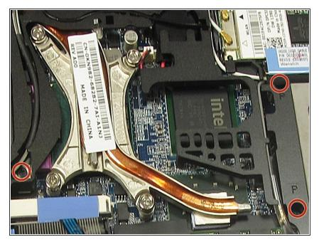
Remove the three (M2.5-8mm) "P" screws indicated to the left and place them in a labeled container.
