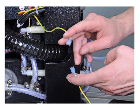
Pull the yellow and green ground wire connectors straight apart to disconnect the bottom cover's ground wire.
