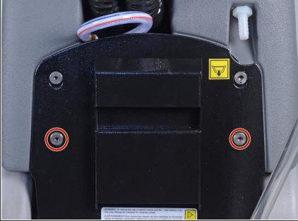
Use a 3 mm hex key to remove two bolts securing the bottom cover.
