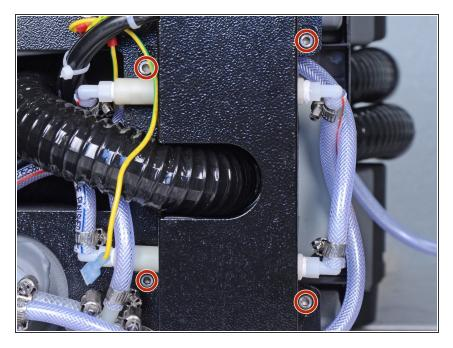
Use a 3 mm hex key to remove the four bolts securing the pump cover.
