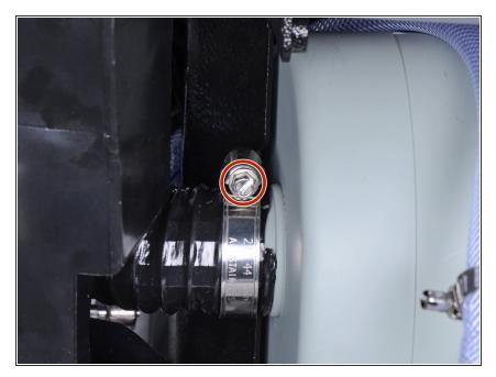
Use a flathead screwdriver to loosen the hose clamp securing the flexible hose to the vacuum motor.
