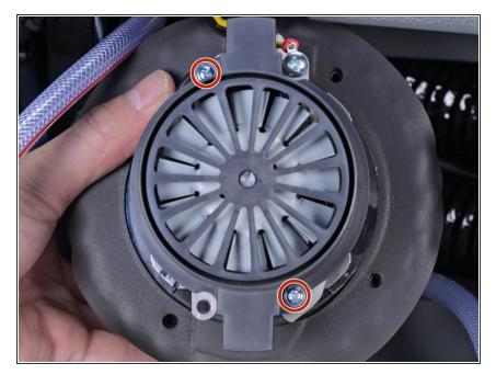
Use a Phillips #2 screwdriver to remove the two screws securing the fan cover.
