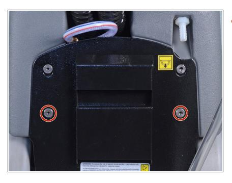
Use a 3 mm hex key to remove two bolts securing the bottom cover.
