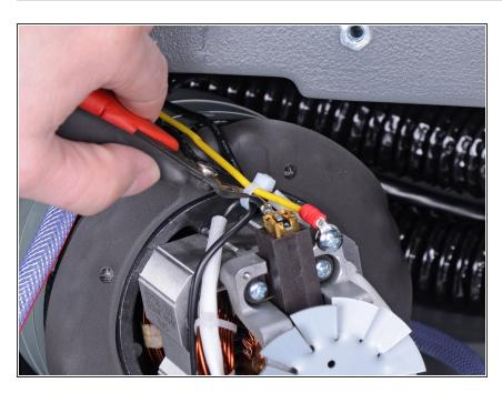
Use a pair of flush cutters to cut all the zip-ties securing any wires to the vacuum motor.
