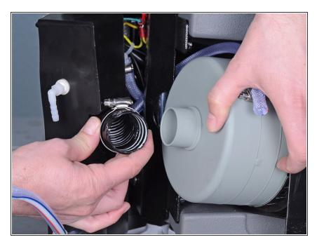
Pull the flexible hose straight off of the vacuum motor to remove it.
