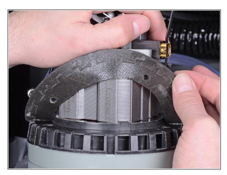
Your new vacuum motor may not come with a vibration damping pad already installed. If so, carefully peel the pad off the old motor and transfer it to the new motor.
