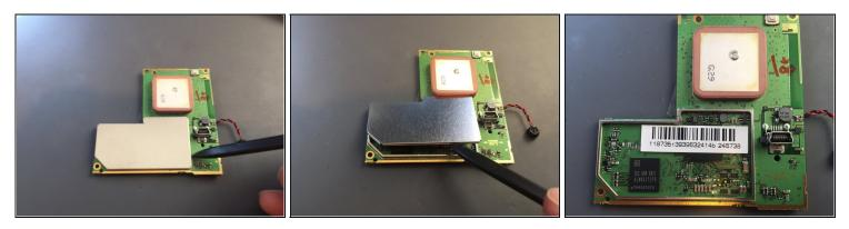
• To reveal all the components, use the spudger to lift off the metal cover of the protected circuitry
