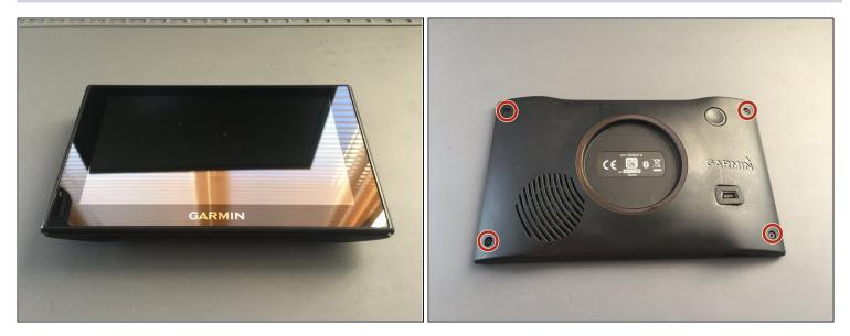
• Turn the device over and remove the 4 x T5 screws.
