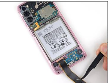
Gently peel up and bend the display flex cable out of the way of the motherboard and battery.
