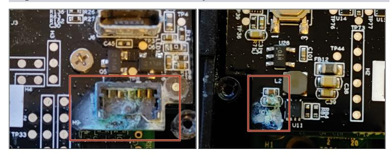
Examine your ring video doorbell motherboard for corrosion on any resistors, capacitors, or battery terminals.
