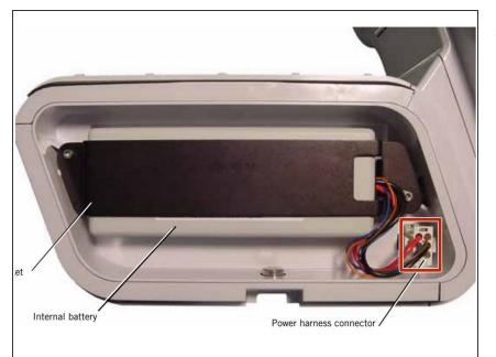
Disconnect the internal battery from the power harness connector.
