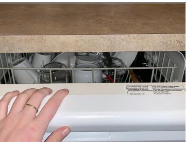
Carefully raise the dishwasher door to align the door latch with the strike plate.
