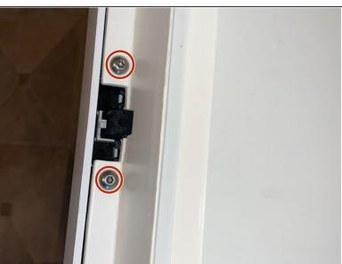
Open the dishwasher door and look for the retaining screws around the side edge and top edge of the dishwasher door.
