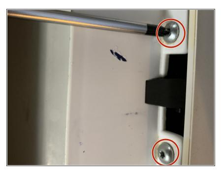
Using a T8 Torx screwdriver remove the two screws by turning counter clockwise.
