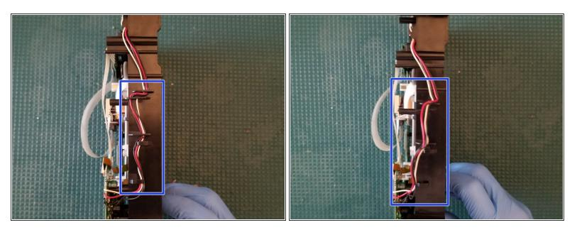
• Loop the wires out from their retaining brackets.
