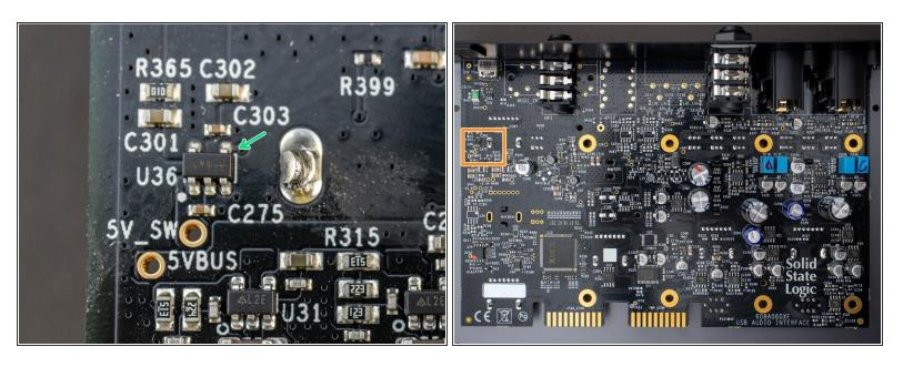
Richtek RT9179 (marked XA9J8) 300mA linear voltage regulator. <u>Data Sheet</u>.
