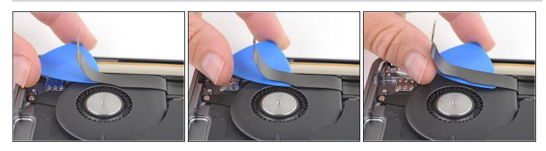
Slide an opening pick under the audio board cable to slice through the adhesive securing it to the fan.
