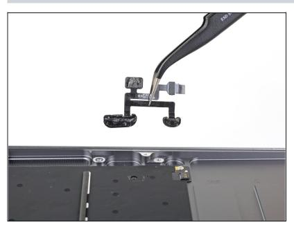
• Remove the microphone assembly.
