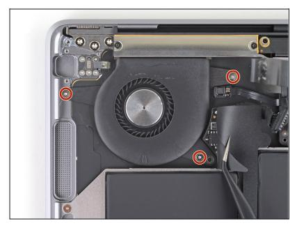
Use a T5 Torx driver to remove the three 2.7 mm screws securing the fan.
