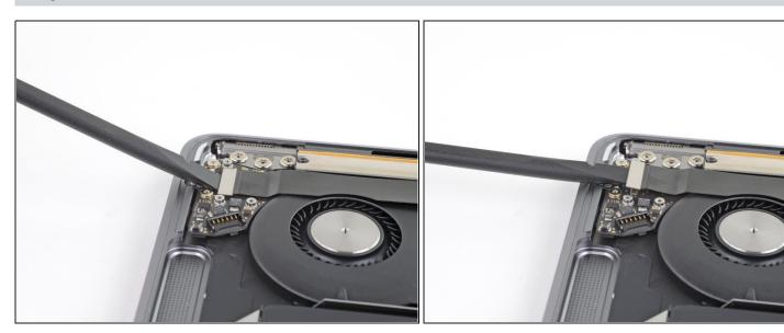
Use the flat end of a spudger to pry the audio board connector straight up and disconnect it.
