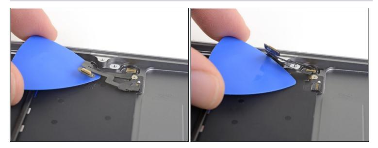
Slide an opening pick under the rest of the microphone assembly cable to separate it from the adhesive securing it to the upper case.
