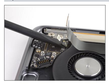
Slide the flat end of a spudger underneath the Touch ID sensor cable to slice through the adhesive securing it to the audio board.
