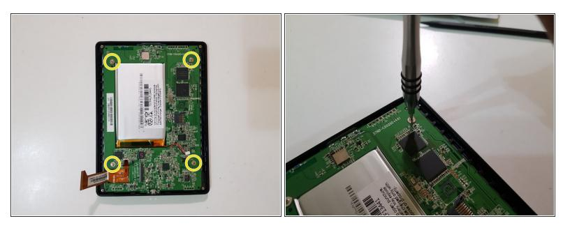
Using your screwdriver with a PH00 tip, remove these screws and set them aside.
