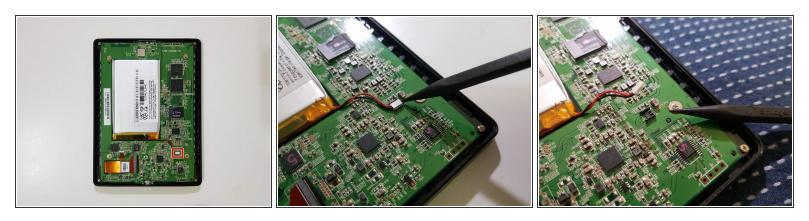
Using the pointed end of your spudger, while holding your eReader using your other hand or a weight, disconnect the battery.
