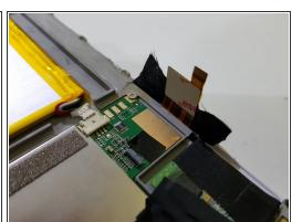
• Using the pointed end of a spudger, disconnect the touch panel.
