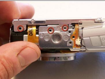
• Remove the three screws attached to the bottom of the LCD brackets
