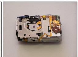
• Lift the LCD screen and remove the two ribbon cables.
