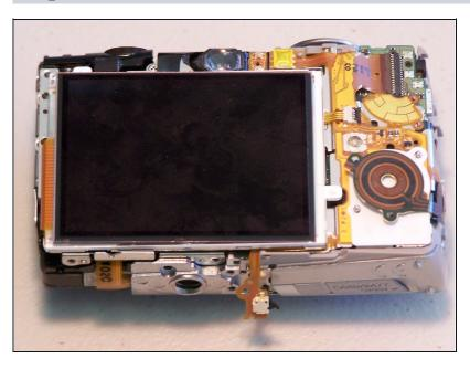
At this point the screen should be easy to lift from the camera body.
