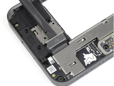
Use a spudger to pry up and disconnect the bottom module connecting cable.
