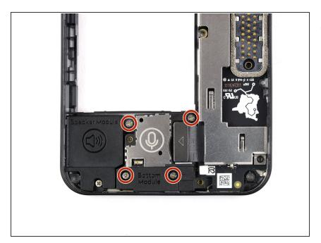
Remove the four 4.1mm-longPhillips #00 screws.
