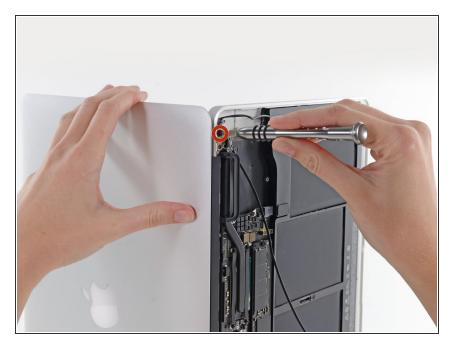
While holding the Air steady, remove the remaining 5.6 mm T8 Torx screw from the left display bracket.
