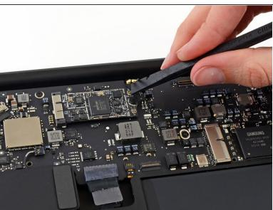
Use the flat end of a spudger to pry each of the antenna connectors up from their sockets on the AirPort/Bluetooth card.
