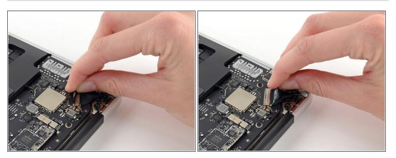
Pull the plastic tab on the display data cable connector to unlock it.
