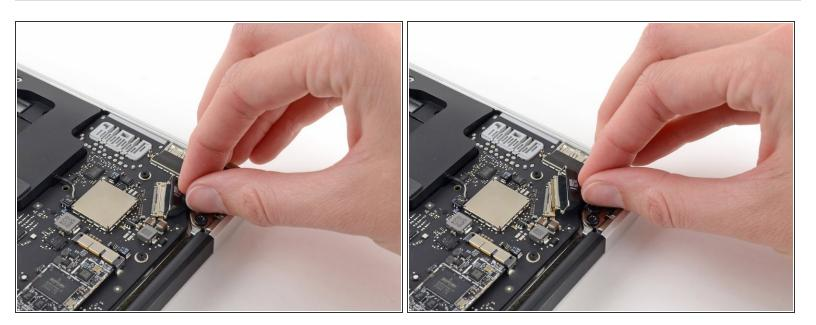
Pull the display data cable connector straight out of its socket.
