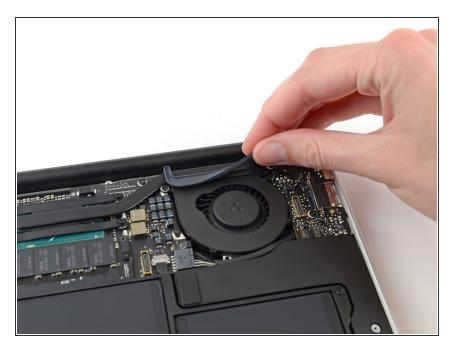
Peel the rubber gasket off the adhesive on the top of the fan.
