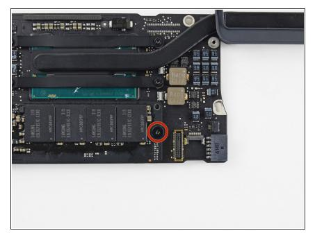
Remove the single 2.85 mm T5 Torx screw securing the SSD to the logic board.
