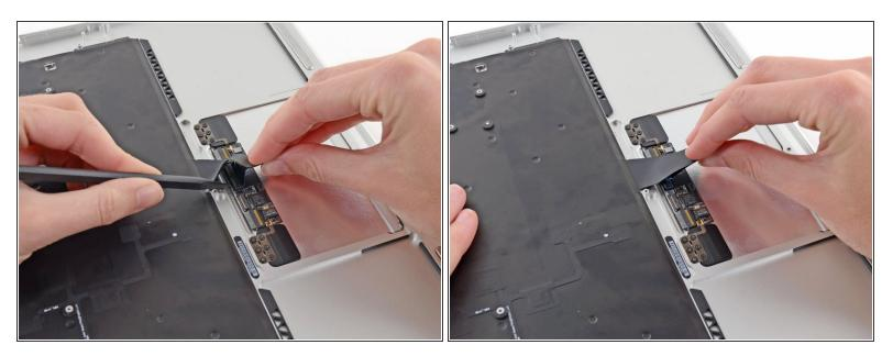
While carefully lifting the keyboard ribbon cable with one hand, use the tip of a spudger or your fingernail to flip up the retaining flap on the keyboard ribbon cable ZIF socket.
