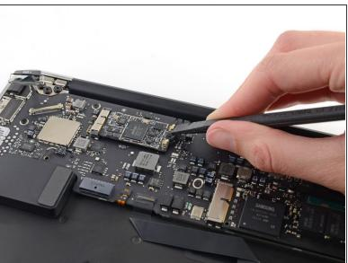
Use the flat end of a spudger to pry both antenna cable connectors up and off their sockets on the AirPort/Bluetooth card.
