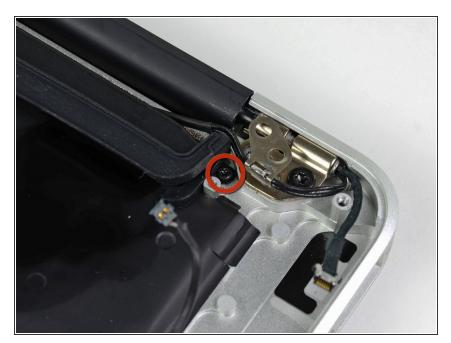
Push the antenna cable retainer away slightly and remove the 3 mm
