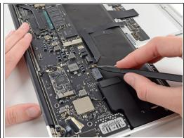
Use the tip of a spudger to flip up the retaining flap on the keyboard backlight ribbon cable ZIF socket.
