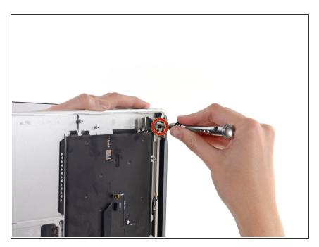
While holding the Air steady, remove the remaining 5.6 mm T8 Torx screw from the display bracket.
