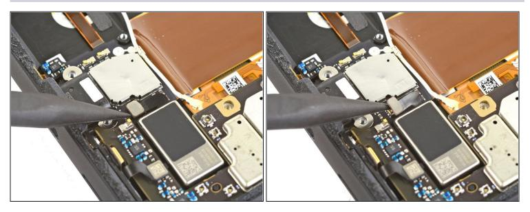
• Disconnect the vibration motor connector from the charging assembly.
