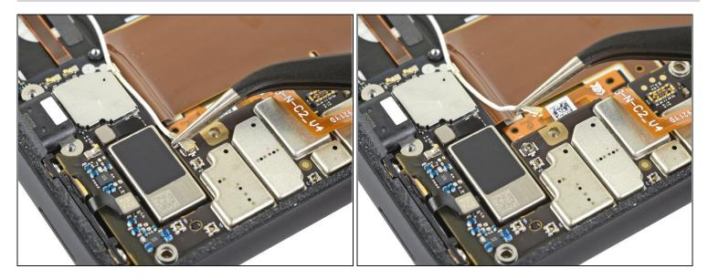
• Use a pair of tweezers to disconnect the <u>antenna press connector</u> from the charging assembly by pulling it straight up from the motherboard.
