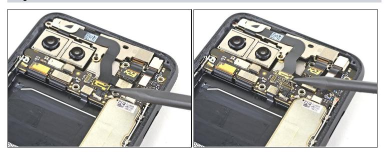
Disconnect the additional sensor connector.
