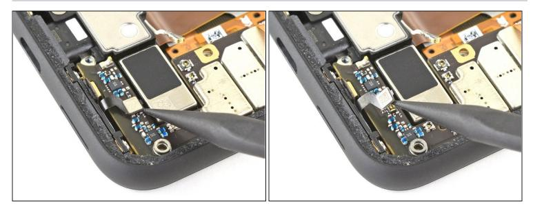
• Disconnect the bottom microphone connector from the motherboard.
