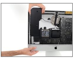
• Lift the left speaker straight up and remove it from the iMac.
