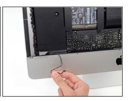
Gently de-route the power button cable from its groove in the left speaker.
