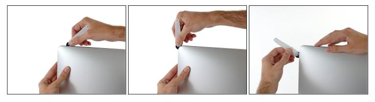
Push the tool around the top right corner of the display.
