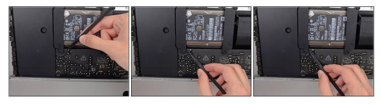
• Use a spudger to disconnect the power button connector from its socket on the logic board.
