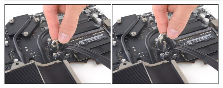
• Pull the PRAM battery straight up and out of its socket.
