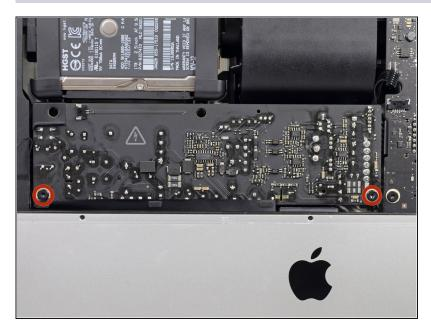
Remove the two 7.2 mm T8 Torx screws securing the power supply to the rear enclosure.
