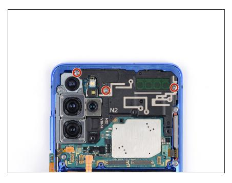
Use a Phillips #00 screwdriver to remove the three 4 mm-long screws securing the upper midframe.
