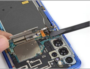
Use a spudger to pry up and disconnect the wireless charging coil connector.
