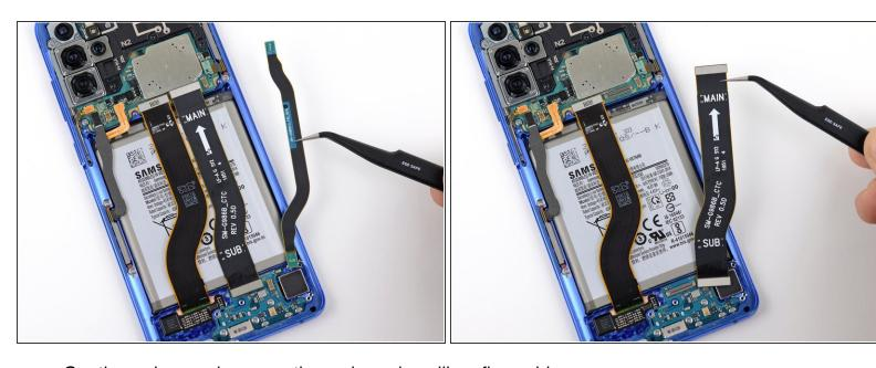
Gently peel up and remove the main and auxiliary flex cables.
