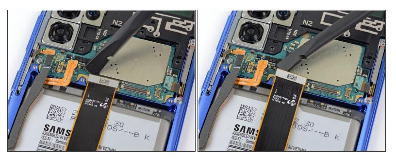
Use a spudger to pry up and disconnect the main display flex cable from the motherboard.
