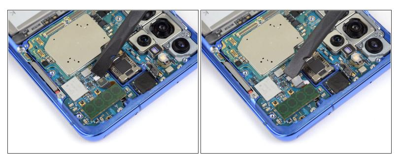
Pry up and disconnect the upper 5G antenna cable from the motherboard.
