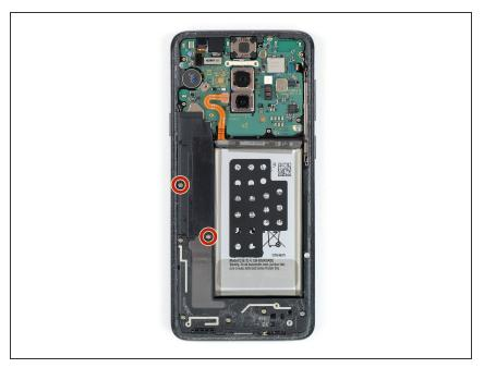
Remove the two 4 mm Phillips #00 screws.
