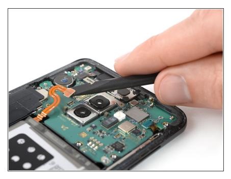
Use the flat end of a spudger to pry up and disconnect the battery flex cable.
