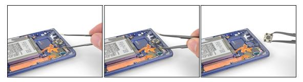
• Insert one side of a pair of angled tweezers into the gap in the side of the phone's earpiece speaker slot.
