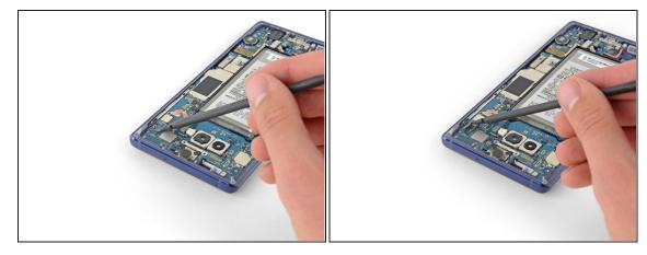
• Use the flat end of a spudger to pry the front sensor connector out of its socket.
