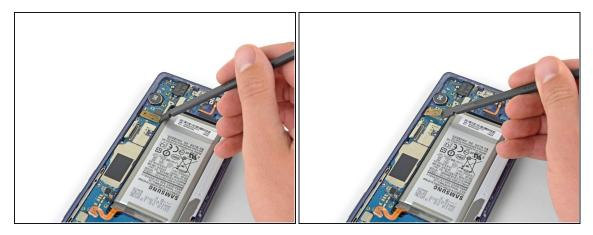
• Use the flat end of a spudger to disconnect the touchscreen cable from the motherboard.
