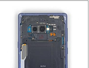
Use a Phillips screwdriver to remove the nine 4 mm screws securing the upper midframe.
