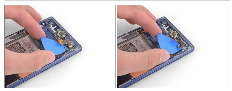
Carefully slide an opening pick under the front sensor array ribbon cable to cut the adhesive underneath.
