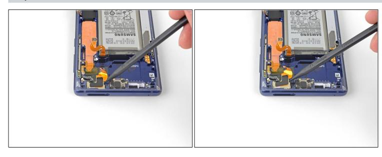
Use the tip of a spudger to lift the left side of the front sensor array and separate the adhesive the rest of the way.
