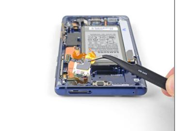
Use a pair of tweezers to remove the front sensor array.
