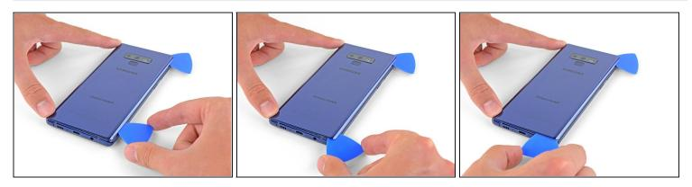
Be careful near the corner, as the glass is very weak. Apply more heat at any time if the adhesive becomes stuck.
