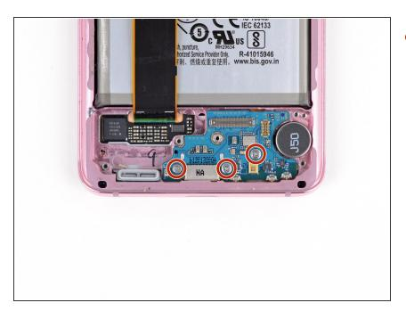
Use a Phillips #00 screwdriver to remove the three 3.4 mm-long screws securing the USB-C port and daughterboard.
