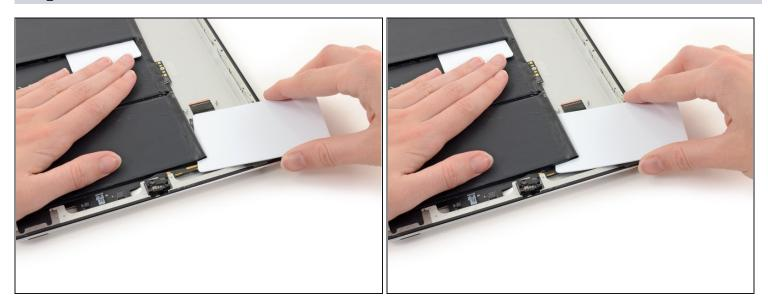
• Slide the card in to free the corner of the cell from adhesive.
