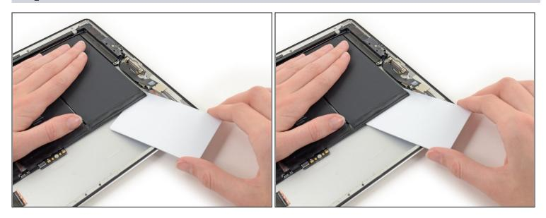
• Insert the card at the case side corner and slide inward to separate more adhesive.
