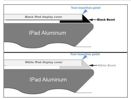
Make sure you place the tool in the proper spot—between the plastic display bezel and the front panel glass.
