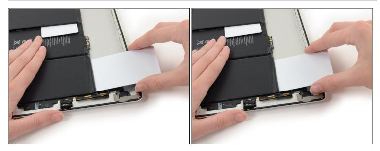
• On the battery cell nearest the headphone jack, run a second plastic card underneath the edge adjacent to the logic board void.
