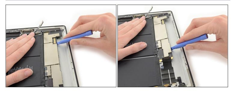
• Use the edge of a plastic opening tool to gently pry the logic board up from the adhesive securing it to the rear case.
