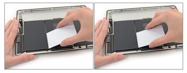
• Gently pry the corner of the battery off of the case to begin freeing the final side of the dock side cell.
