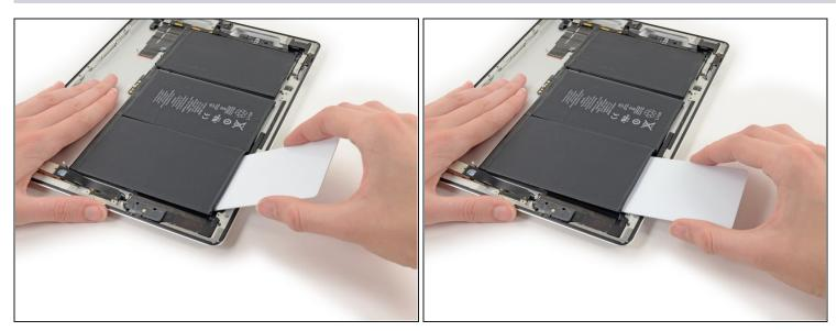
• Gently pry the end of the battery cell away from the case.
