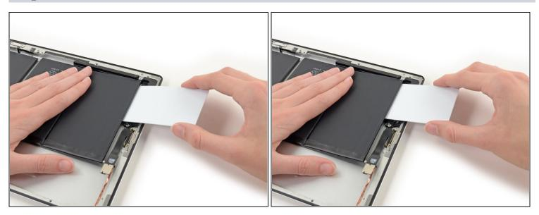
• Insert the card at the bottom corner (closest to the headphone jack) to free this side of the battery cell.
