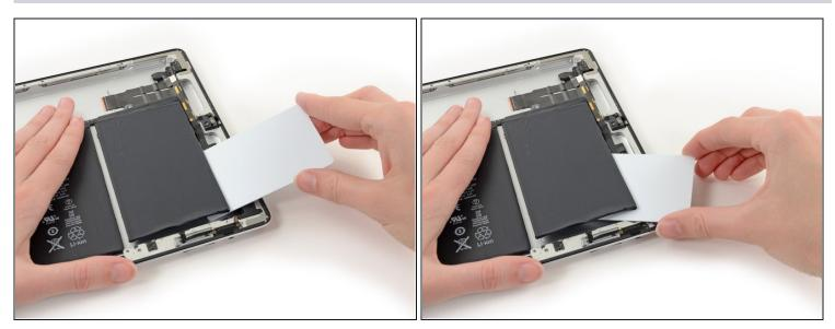
• A final pry, and the card can be left in place to keep the battery propped away from the adhesive.
