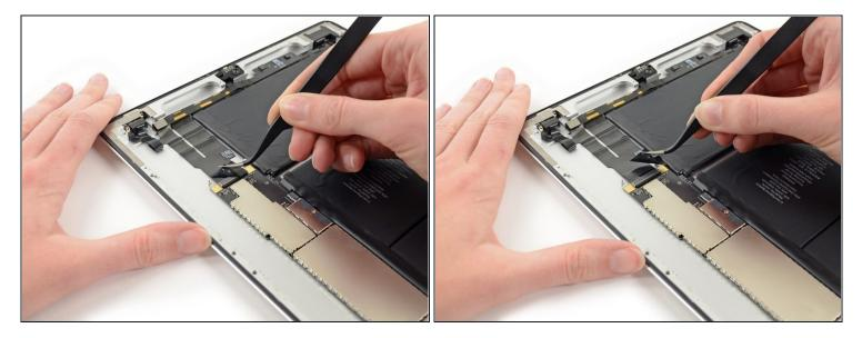
• If present, use tweezers to remove the piece of tape covering the end of the headphone jack/control board cable.
