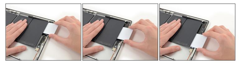
• Slide the card along the side of the cell to detach any remaining adhesive.
