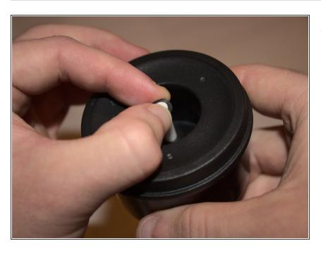
Install the first new thrust washer to the bottom of the ceramic shaft.
