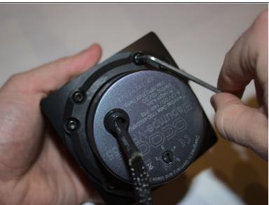
Remove the eight 3.5 cm M4 hex screws securing the pump to the shroud.
