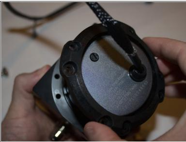
Place the pump into the bottom of the shroud and reposition the tension ring.
