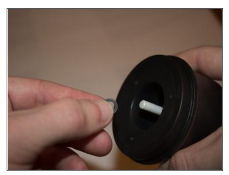
Remove the black lower thrust washer to complete the disassembly.
