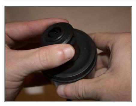
Install the impeller back onto the ceramic shaft on top of the bottom thrust washer.
