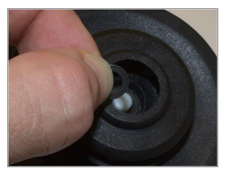
Install the new top thrust washer onto the ceramic shaft.
