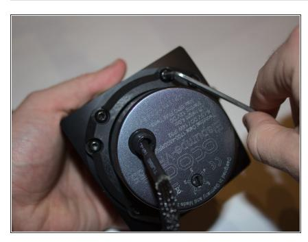
Screw in the eight 3.5 cm M4 hex screws to complete the reassembly.
