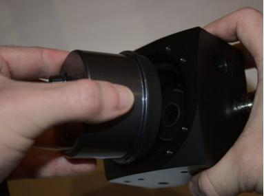
Remove the tension ring and separate the pump from the shroud.
