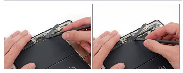
• Use the flat end of a spudger to gently peel up the Lightning connector cable from the aluminum frame.
