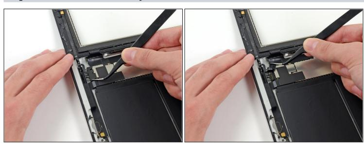
(i) If present, remove the piece of electrical tape covering the Wi-Fi antenna, speaker cable, and home button ribbon cable.
