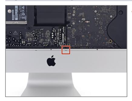
To avoid blocking the microphone port with adhesive, strip 4R must be modified before use. A small notch must be cut out of the lower edge of the adhesive strip to accommodate the microphones.
