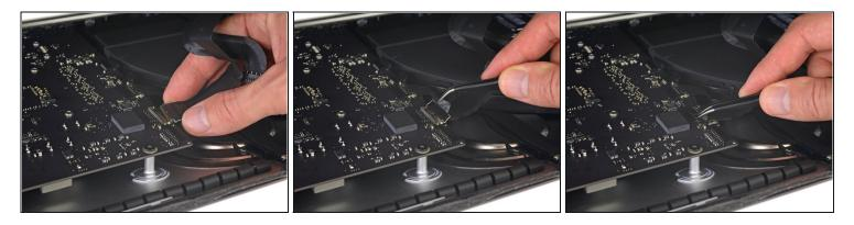
• Use a pair of tweezers or your other hand to gently insert the display data cable connector into its socket on the logic board.
