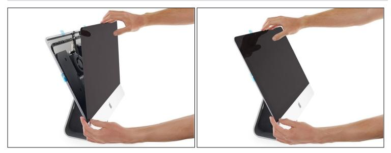
• Gently set the display in place over the iMac and align it carefully.
