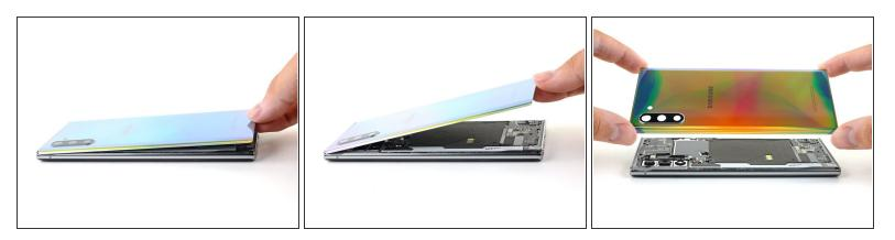
• Lift up and remove the back panel.
