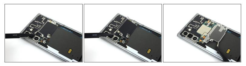
• Use a pair of tweezers to lift up and flip back the metal shield covering the battery connector.
