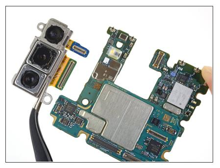
• Remove the rear camera module.
