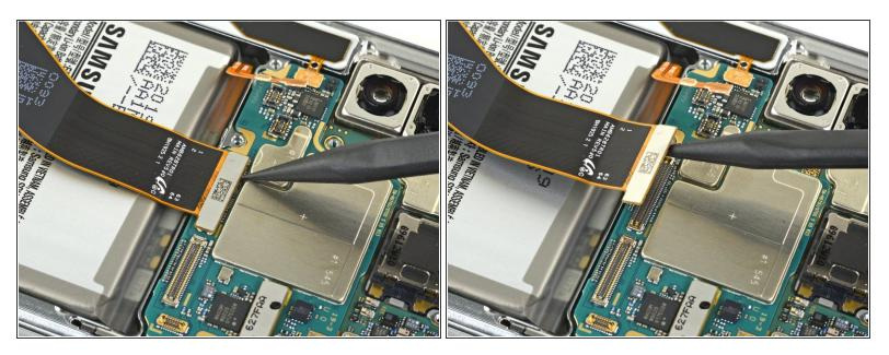
• Use the pointed end of a spudger to disconnect the display cable from the motherboard.
