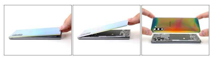
Lift up and remove the back panel.
