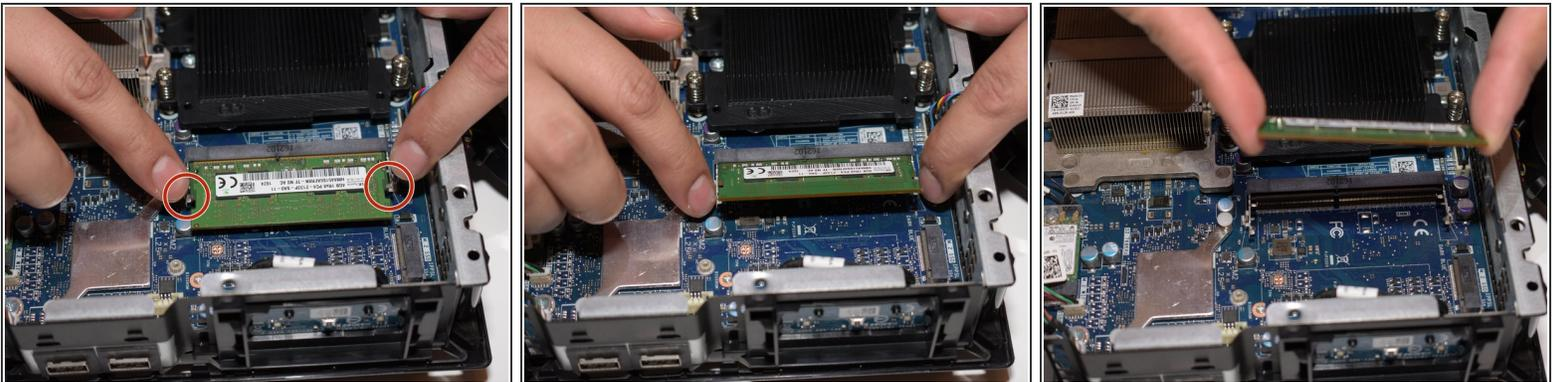
**⚠** Installing the SSD card without removing the RAM could cause grinding of the edges between the RAM and SSD, resulting in damaged components. However, it is possible to skip this step and move straight to the SSD installation.
