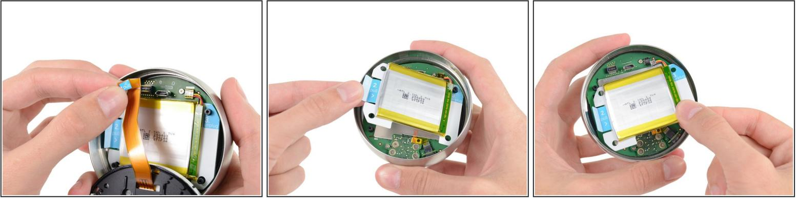
**i** Nothing makes us happier than a device with an [easily replaceable battery](#). We feel the engineers at Nest Labs must have been thinking of us when they added these numbered flags showing three easy steps for battery removal.
