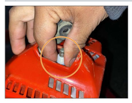
Insert the new spark plug and twist it in a clockwise motion until it is tight.
