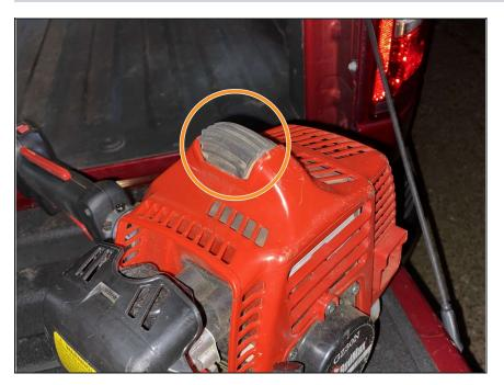
Look for the black plastic cover with ridges on the top of the brush cutter. Your fingers should be enough to pull the plastic off, but you may use a flat head screwdriver instead.
