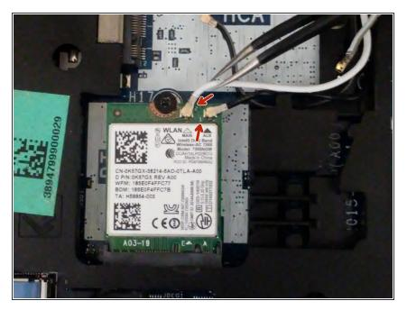
If the wires are not clearly labeled as 1 and 2, take note of how the wires are connected to know which is 1 and 2. The WiFi card should have a tiny 1 and 2 on the card itself for guidance.
