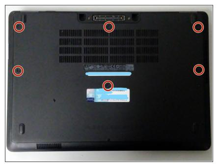
• Remove the 6 screws using a Philips #1 (PH1) screwdriver.
