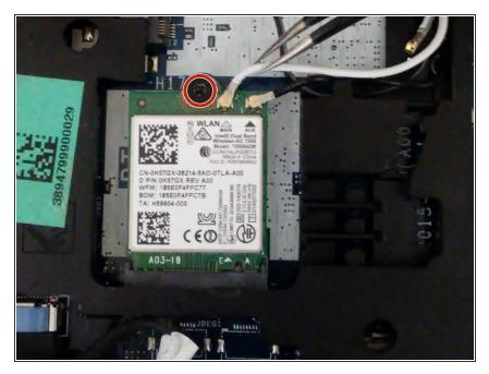
Use a Philips #1 (PH1) screwdriver to remove the screw holding the WiFi card in place.
