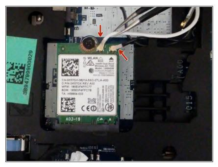
• Gently disconnect the antennas and slide the WiFi card from the slot
